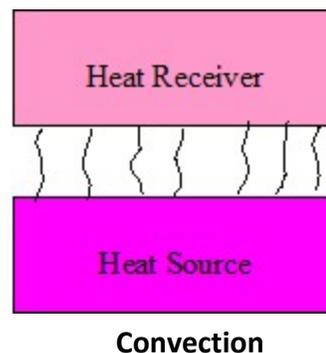
Convective heating relies on the movement of hot fluid or gas, such as air, which acts as a carrier of heat from one body to another. In industry, forced convection is commonly used, that is, the gas or liquid is directed towards the article by a fan or pump. Natural convection occurs because gas or liquid at different temperatures have different densities. An ordinary central heating radiator emits heat mainly through "natural convection".
